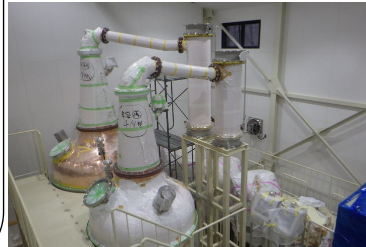
Pot stills for first (in back) and second (front) distillation
